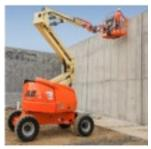
Articulating Boom Aerial Lift This aerial lift has at least 2 hinged sections which are used to increase mobility.
