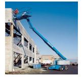
**Extendable / Telescoping Aerial Lift** This aerial lift has a boom that extends horizontally and vertically.
